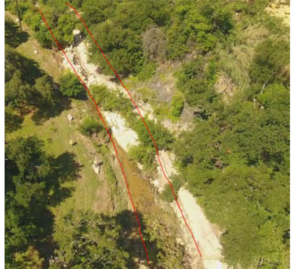
Top view of trail at creek, along toe of slide looking d/s Rough approximation of pre-event creek bottom width (shown by red line)
