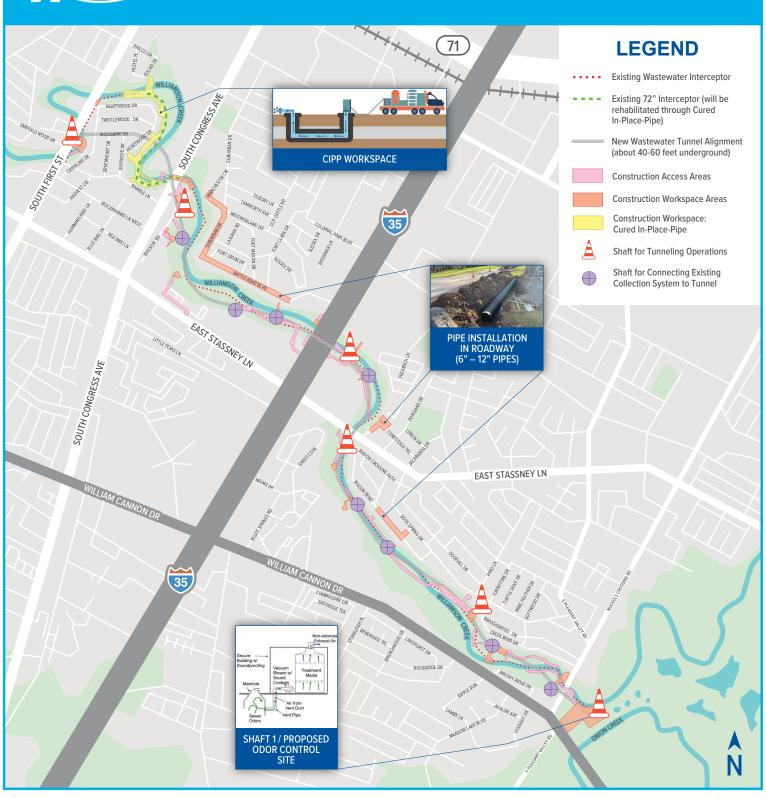
**Wastewater Interceptor:** A major pipeline that receives wastewater flows from collector lines and carries it to a treatment facility. The Williamson Creek Interceptor carries wastewater to the South Regional Treatment Facility.
