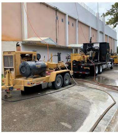
Water is pressurized with dieselpowered pumps (up to 4 running at a time)
