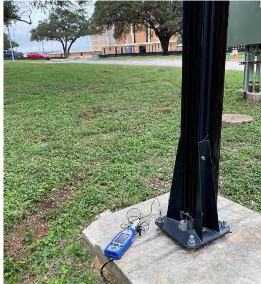
Figure 3-3: Example of Ground Vibration Measurement Equipment Setup
