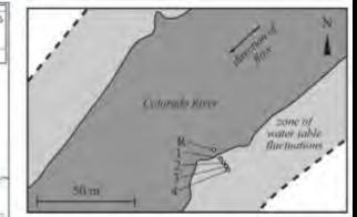
Figure 2: Map of Hornsby Bend piezometer transect. Bank piezometers are numbered in order of distance from the river, and the river stage recorder is denoted as (R). Dashed lines indicate the estimated extent of dam influence on the water table.
