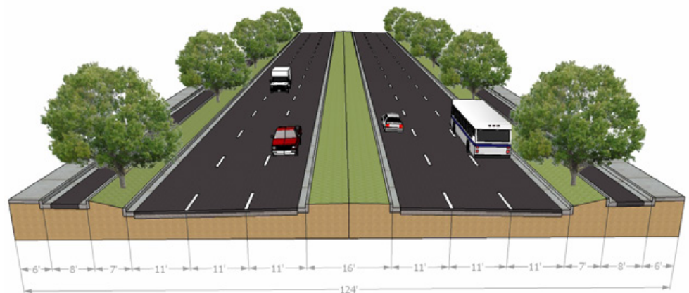
FIGURE 2 – US 183 to Decker Lane (FM 3177) – Ultimate Typical Section
