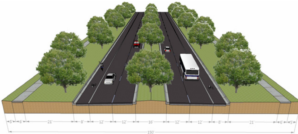
FIGURE 41 – FM 973 to Dunlap Road – 2025 Typical Section
