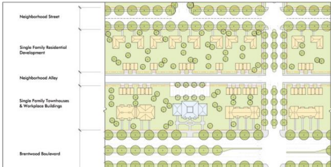
Figure 24. A neighborhood-oriented vision for corridor segments: At the boulevard, “mansion-scale” homes and workplace buildings mix compatibly due to similar scale and style. To the rear, alleyway circulation to locate parking, leaving the streets and home frontages safer and more attractive. 26
