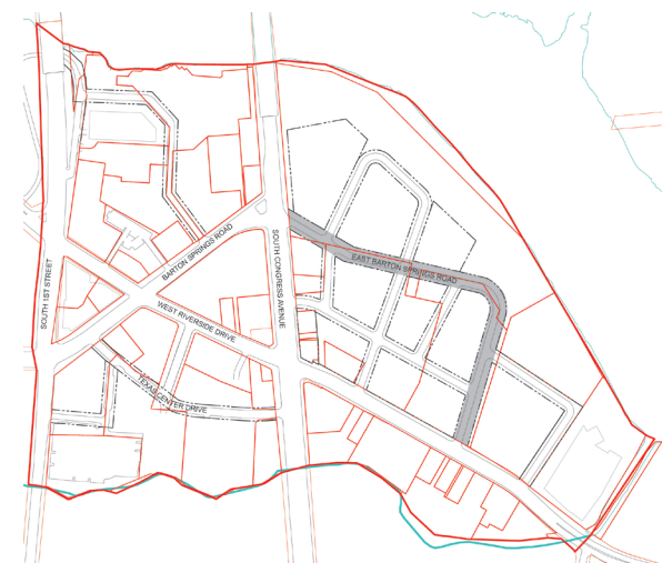
Figure 3: Possible Alignments of Barton Springs Road Extension
