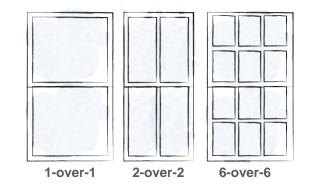
**Above:** The window type and number of lites, or panes of glass, in a window speak to a building's construction period and architectural style. Early windows are typically 1-over-1 or 2-over-2 double-hung wood-sash windows; the 6-over-6 lite pattern appeared in the 1930s and 40s. Sometimes window screens added ornamentation by making windows appear to contain more lites.
