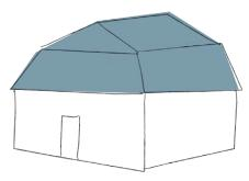
Mansard roof A roof with two slopes on all four sides; the lower slope is steeper than the upper.
