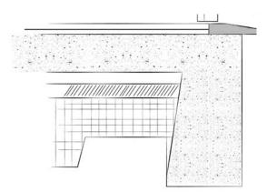
**Concrete slab foundation**
