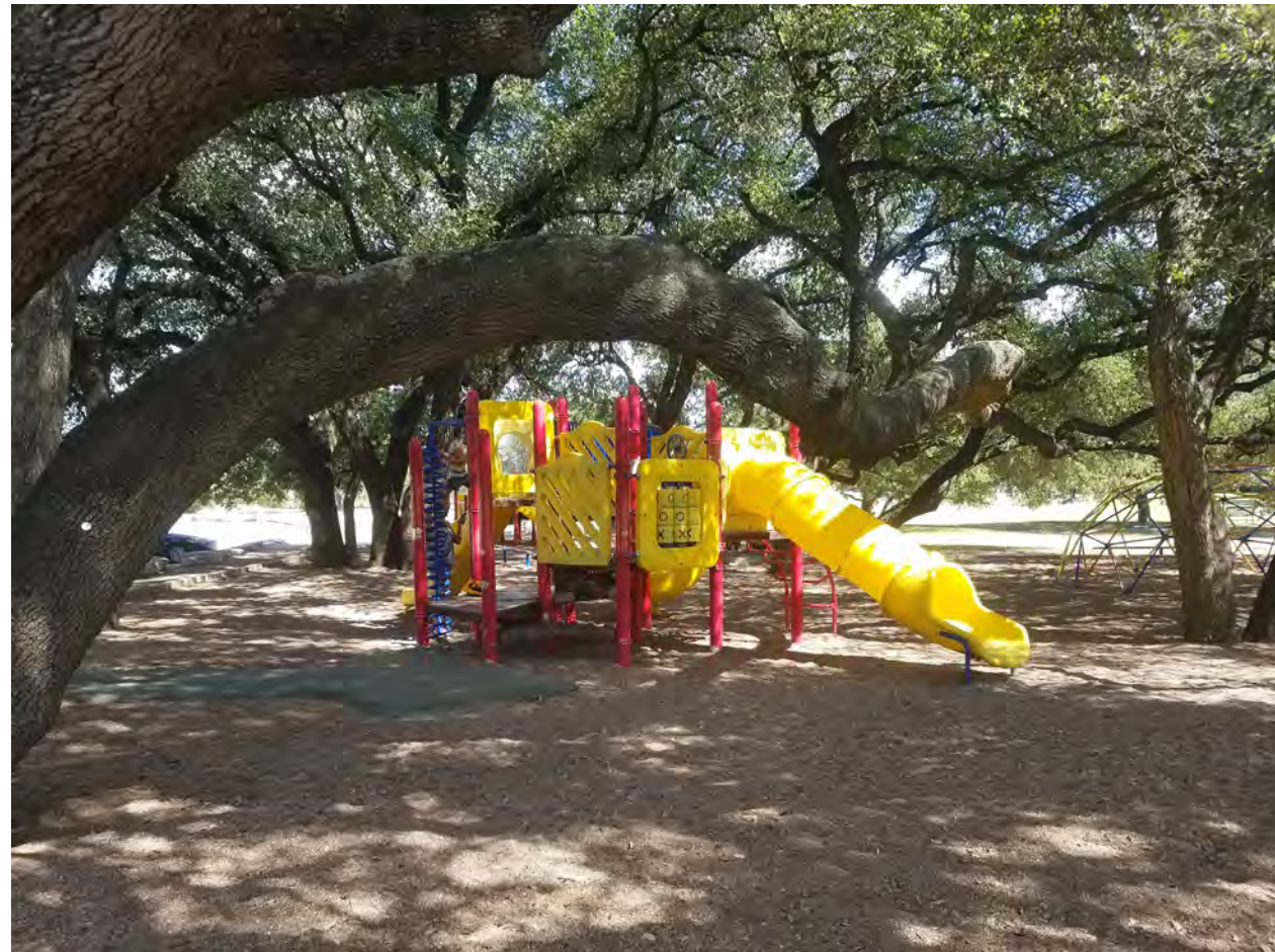
NO ACCESSIBLE PLAY OPTIONS AT EXISTING LOCATION. IF PEAGRAVEL WERE REPLACED WITH 12" DEEP SAFETY MULCH IT COULD CAUSE ROT AND MOISTURE DAMAGE AT THE BASE OF THE TREE TRUNKS
