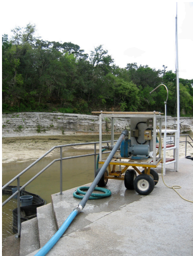
Trash pump used for silt disposal.
