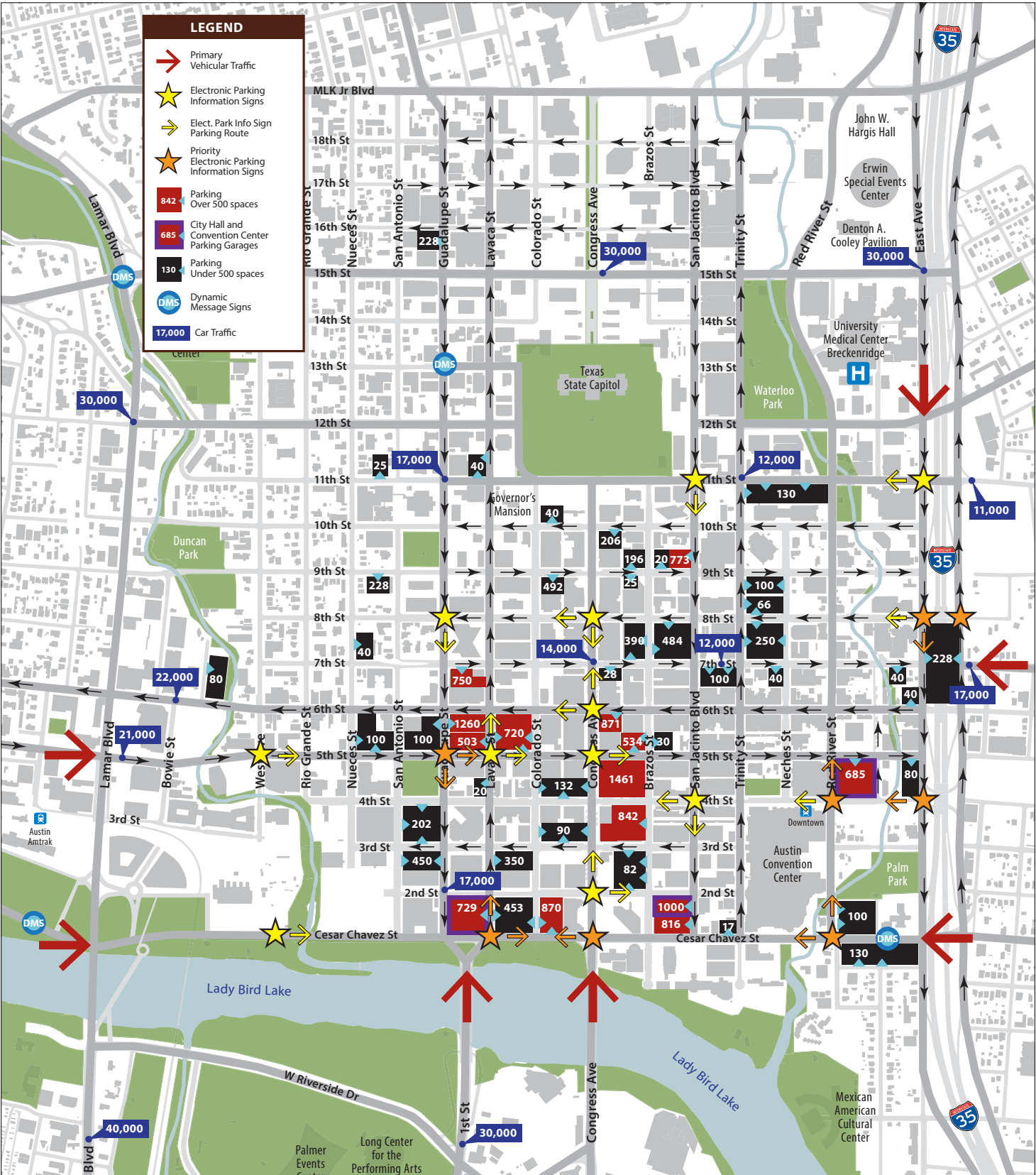
FIGURE 3.18 Map shows available parking spaces and car traffic at various entry and exit roads. Final locations of electronic parking signs shall be based on traffic study from ATD.
