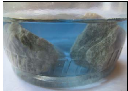
The water will eventually turn blue to indicate basic pH
