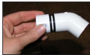
Same picture as above with another #18 O-Ring and the ¾" 45° elbow added. Note: the coupler and one O-Ring should be on the inside of the container and the other O-Ring and ¾" 45° elbow should be on the outside of the container. All parts should be pressed together tightly to make a watertight seal.
