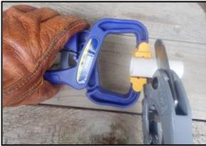
Wear leather gloves and use a clamp to hold the PVC or PVC coupler while using the ratcheting PVC cutter
