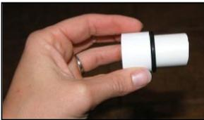
¾" PVC tubing with #18 O-Ring (black) and coupler cut in half (on left).
