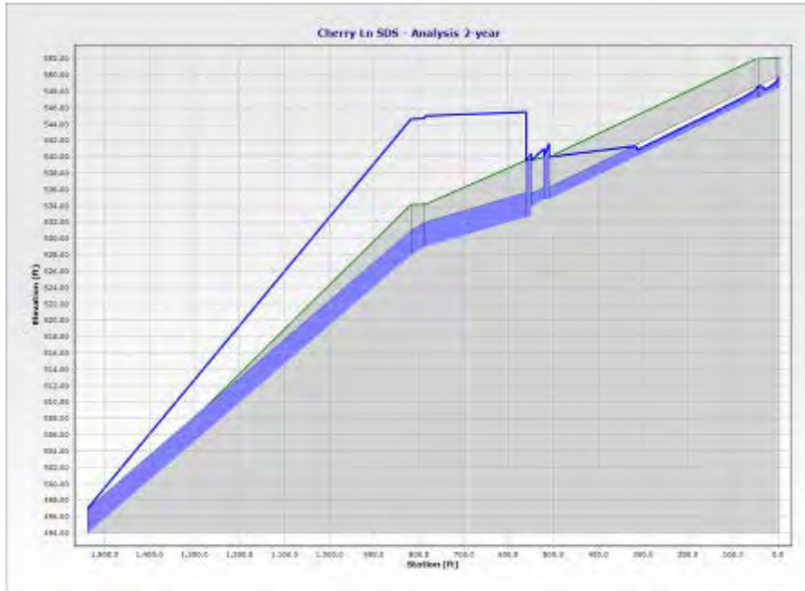
Figure 10. Cherry Storm Drain System Main Trunk, 2-year storm profile
