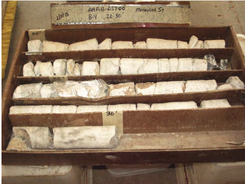
Photograph 15 – Boring B-4 – Depths 20'–30'
