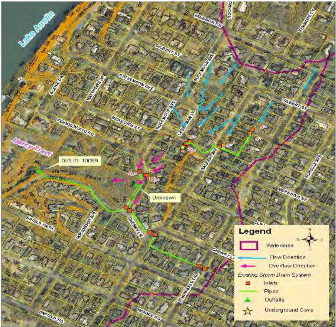
Figure 3. Existing Storm Drain Systems in Project Area: Meredith SDS (upper) and Cherry SDS (lower), NTS
