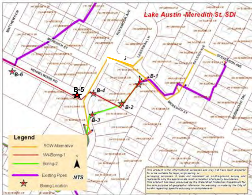
Figure 1. Site map showing Meredith Street and Rockmoor Avenue and borehole locations (Raba Kistner Consultants, Inc.). Borehole locations B-1 through B-5 approximately defines the boundaries of the quarry operation that took place in early 1900s. Sinkholes and caves were observed during the quarrying of the Edwards Limestone. Edwards Limestone, Georgetown Limestone and Del Rio Clay still outcrop in and around the site.
