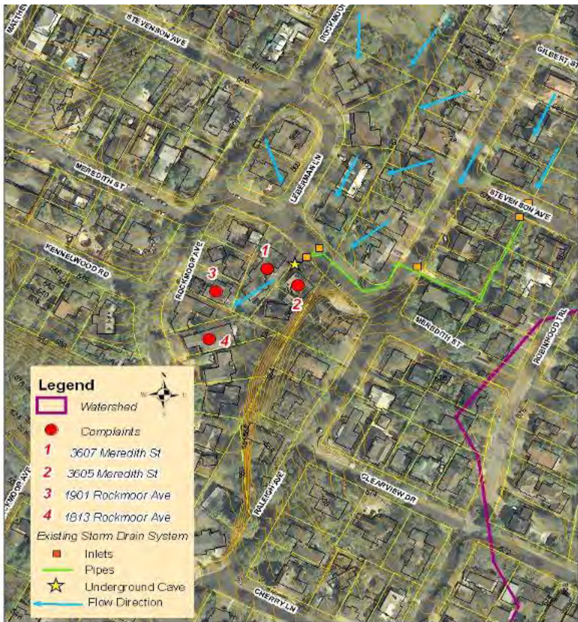
Figure 2. Meredith St. Complaints and Existing Storm Drain (Meredith SDS), Not To Scale (NTS)
