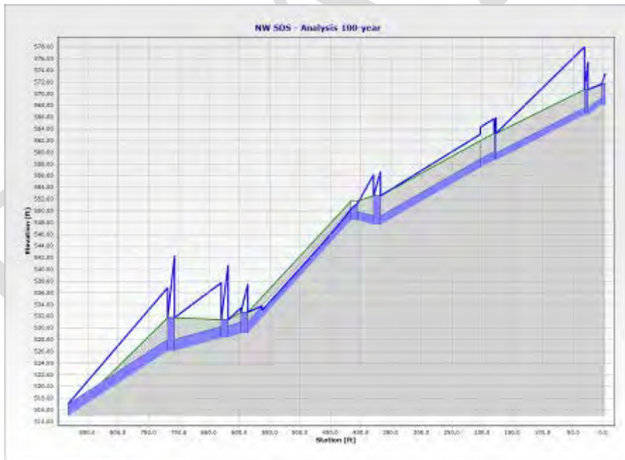
Figure 9. NW Storm Drain System Main Trunk, 100-year storm profile
