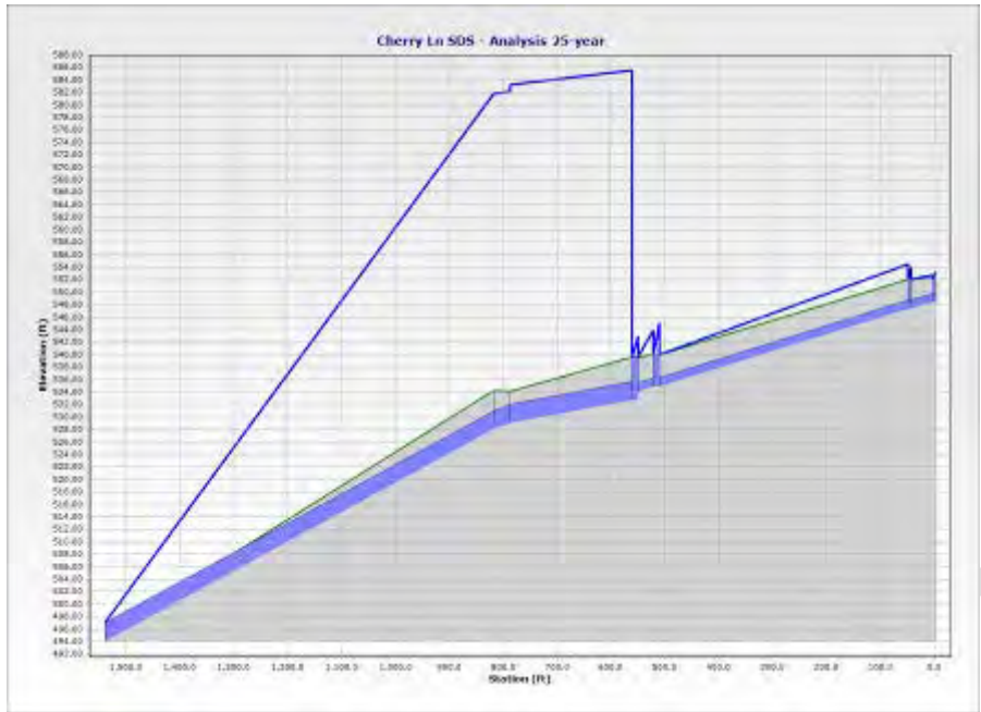
Figure 12. Cherry Storm Drain System Main Trunk, 25-year storm profile
