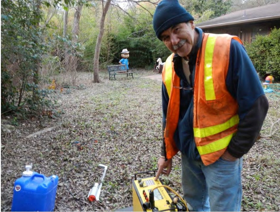
Picture 3. Taking resistivity survey along profile G2. The recording resistivity unit was set in the backyard of 3605 B Meredith Street. There are rocks outcropping to the east, which appear to be Georgetown Limestone.
