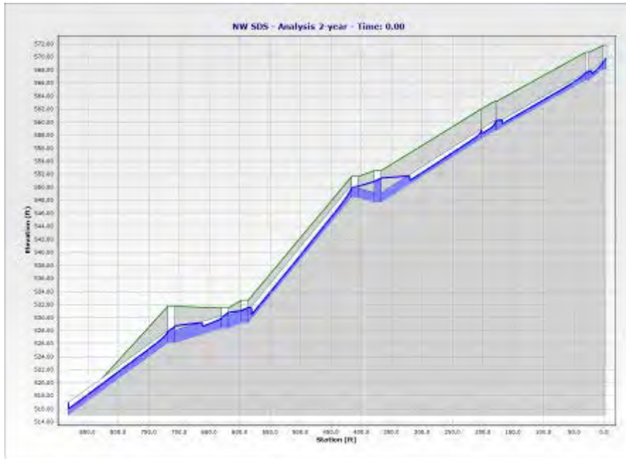
Figure 6. NW Storm Drain System Main Trunk, 2-year storm profile
