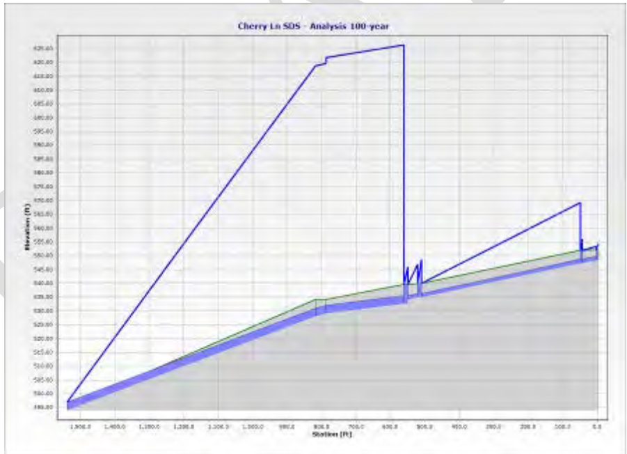
Figure 13. Cherry Storm Drain System Main Trunk, 100-year storm profile
