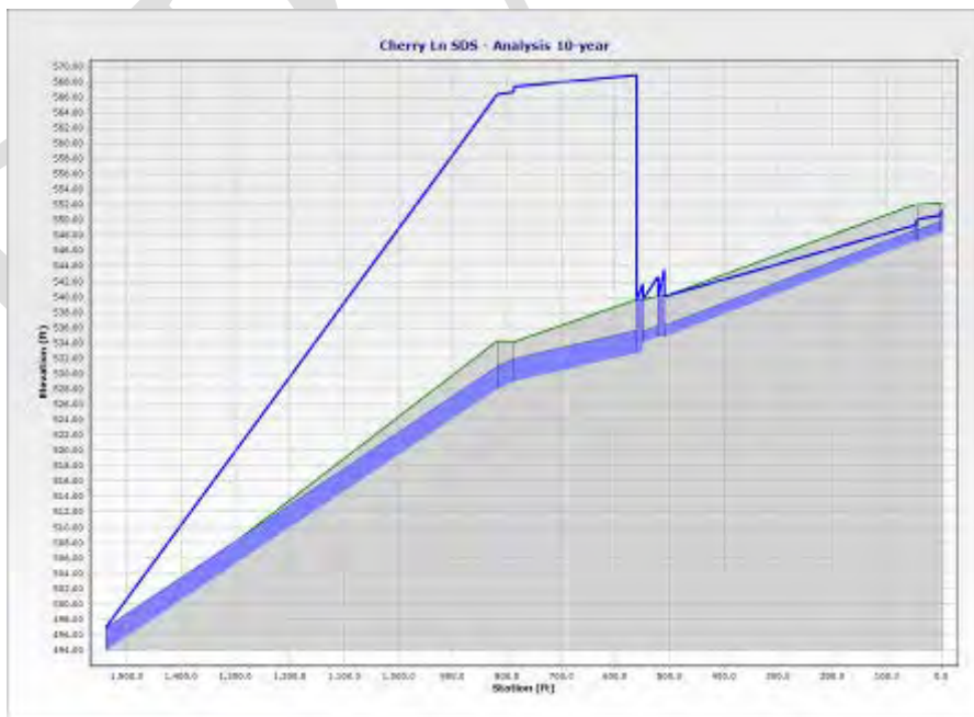
Figure 11. Cherry Storm Drain System Main Trunk, 10-year storm profile
