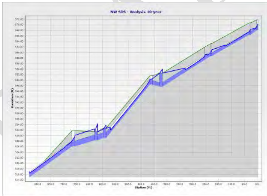
Figure 7. NW Storm Drain System Main Trunk, 10-year storm profile
