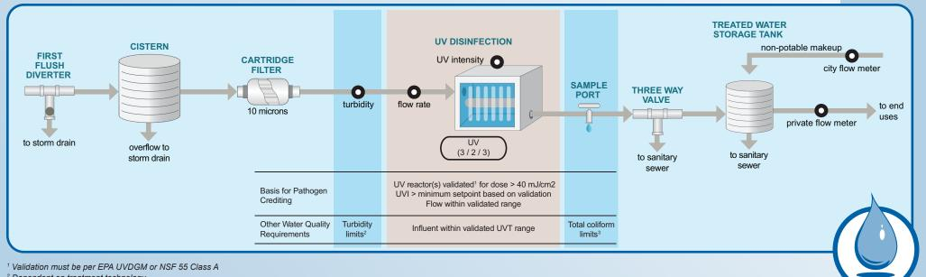
For rainwater, the only specified LRT is for protozoa. In this example, the LRTs are met with a validated UV reactor that operates within certain operating conditions. The inclusion of a cartridge filter upstream of the UV reactor provides pre-treatment to improve the water quality of the water prior to disinfection and helps meet the turbitidity limits. Because the use is outdoors, no chlorine residual is required.
