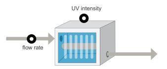
With the UV Intensity Setpoint approach, UVT monitoring is not required on the influent to the UV reactor. However, it is critical to consider the likely water quality of the influent in terms of UVT when selecting the appropriate reactor. An MBR-treated blackwater may have a UVT in the 60-75% range; if a reactor was validated only down to a UVT of 80%, the system will fail to meet the UV intensity setpoint and thus the reactor would not be an appropriate choice.
