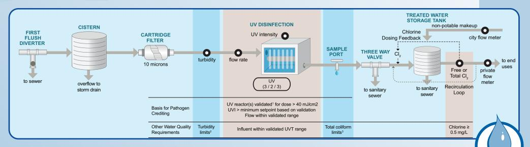
For rainwater, the only specified LRT is for protozoa. In this example, the LRTs are met with a validated UV reactor that operates within certain operating conditions. The inclusion of a cartridge filter upstream of the UV reactor provides pre-treatment to improve the water quality of the water prior to disinfection and helps meet the turbitidity limits. Because the use is indoors, a chlorine residual is required.
