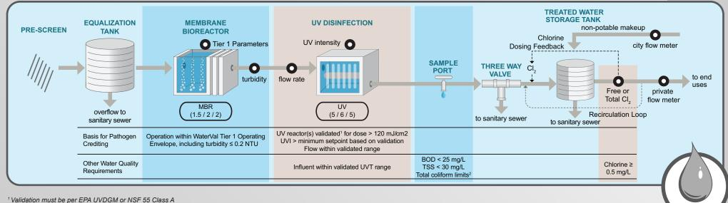
In this example, the graywater system meets the LRTs for indoor use using MBR and UV:
