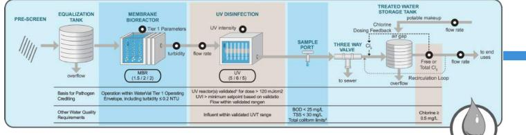
Figure 4. Example Reuse Technologies for Scenario 2: Graywater storage and treatment components. Image: Austin Wate
