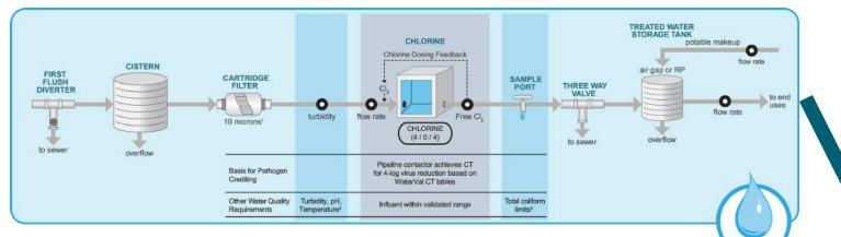
Figure 3. Example Reuse Technologies for Scenario 1: Rainwater harvesting storage and treatment components. Image: Austin Water
