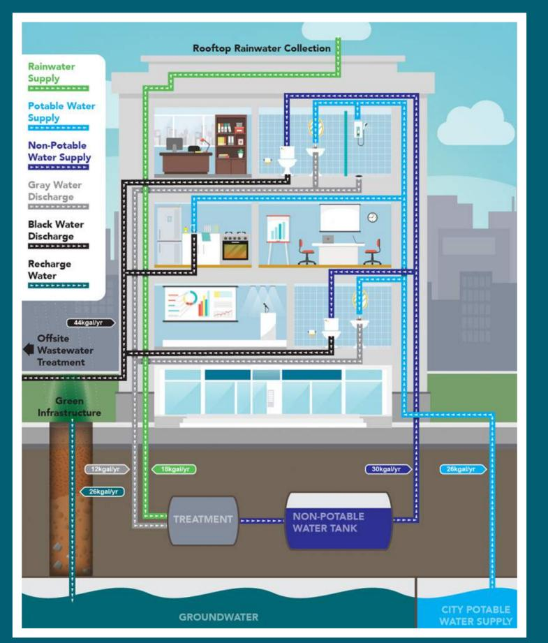
Figure 1. An illustration of the types of water available for reuse in a building. Source: Office of Energy Efficiency & Renewable Energy. Available at <u>energy.gov/eere/femp/scenario-2-mainstream-net-zero-water-building</u>.
