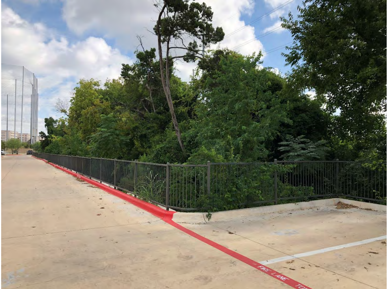
Image 11: Roughly 17' deep wetland (identified on site as Grow Zone) along the Esperanza Crossing apartment's property line is adjacent to the CapMetro tracks. Wetland at its widest is 65' wide and narrows down to roughly 10' wide, which will need to be a pinch point for the trail. Additionally, the trail will need to be up against the apartment's retaining wall.
