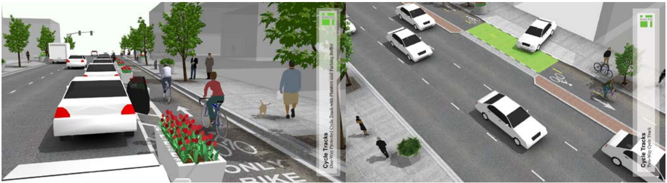
Caption: One-way and two-way protected bicycle lanes as shown in the NACTO Urban Bikeway Design guide (Graphic courtesy of NACTO, Urban Bikeway Design Guide)
