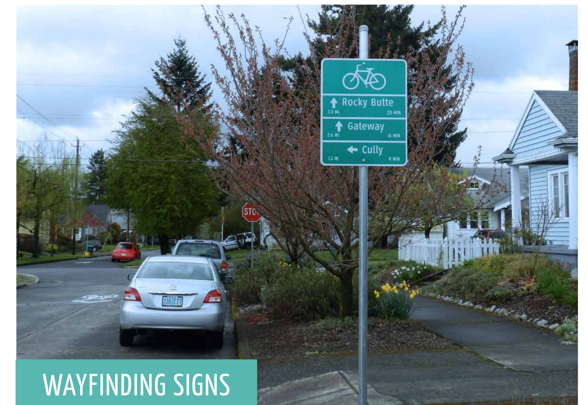
Wayfinding signs help to guide people along the bikeway route to local and regional destinations. Wayfinding signs can include information on the distance and approximate time it takes to bicycle to a destination. Photo: Portland, Oregon
