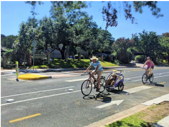
Example of pedestrian crossing islands and a two-way protected bikeway constructed using concrete traffic buttons and planters on Barton Hills Drive
